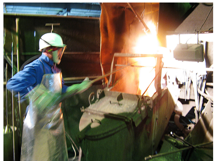
Fig. 6: An employee of Weser-Metall measures the temperature at the slag tick of the immersion melting furnace.
