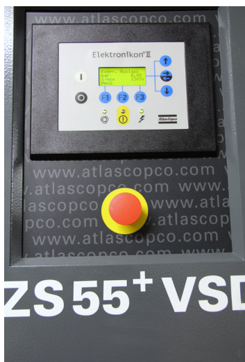
Fig. 3: The ZS+ screw blower is supplied by Atlas Copco as a complete package, ready for operation, with PLC-based electronic control unit, integrated inverter, and much more.
